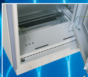
Cabinet bottom with pivot frame crossbar and flexible cable entry via foam rubber
